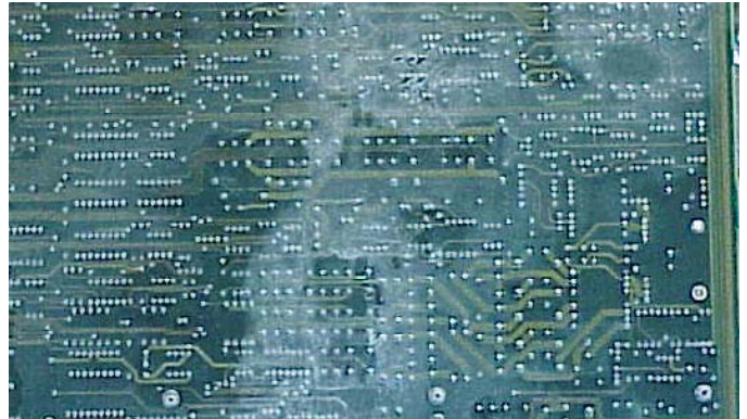
Figure 1: white residue from no clean flux hand soldering
