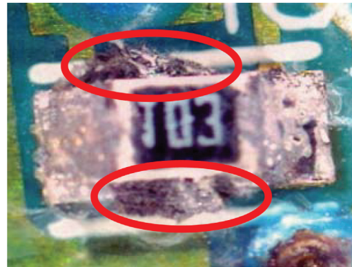
Photo 1 – Electrochemical migration occurring due to high levels of water soluble flux residues left on the board
