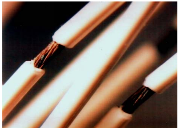
Photo 2: Corrosion Under Teflon Insulation
