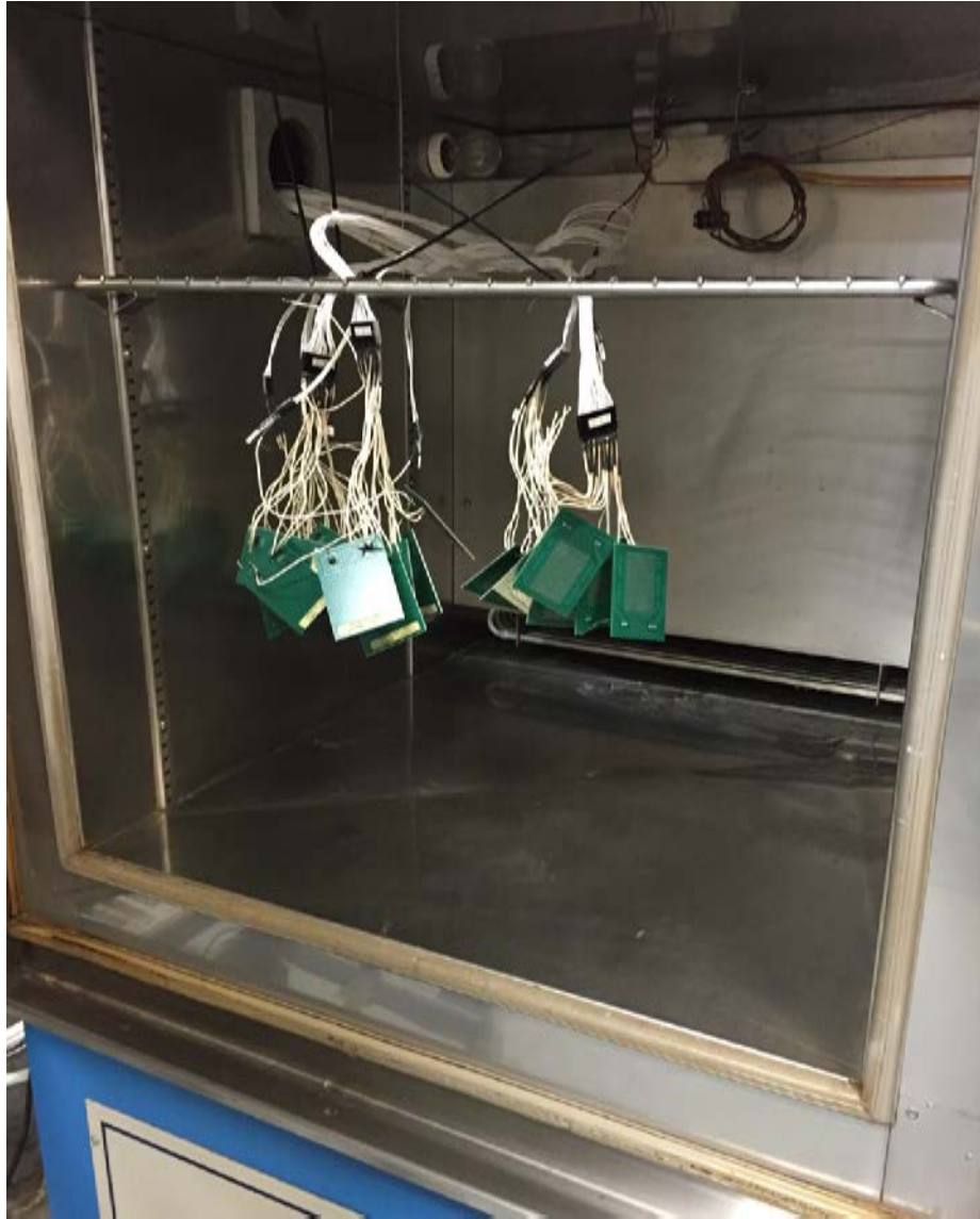
Figure 2: SIR coupons in chamber before the start of testing
