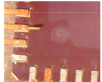
LCC area with heavy water soluble flux residues trapped under the 5 mil standoff of the 68pin LCC.
