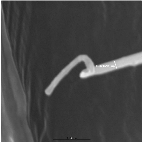
Figure 9 – SEM of whiskers removed from capacitor
