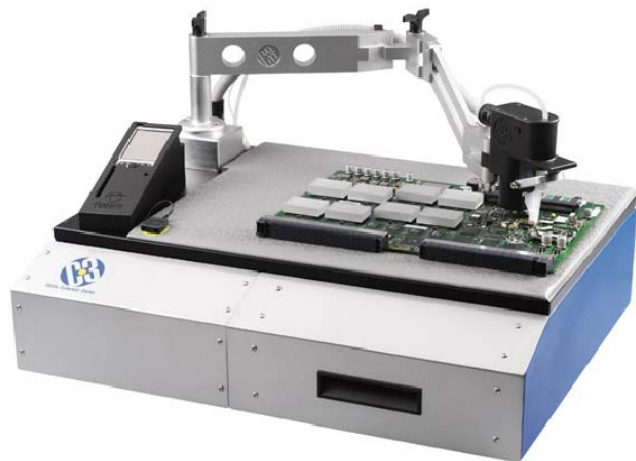
Figure 12 – C3 test system for localized extractions
