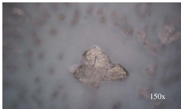
Figure 5 – Inside ESD bag surface above capacitor #2
