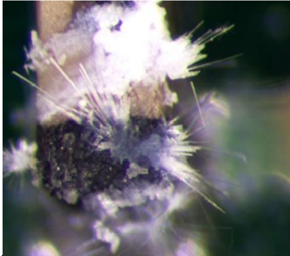
Figure 3 – Capacitor #1 with tin whiskers on power input side
