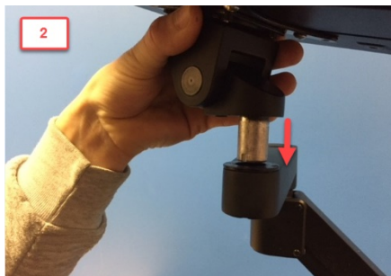
Attach tray to arm and attach washer under arm to tray
