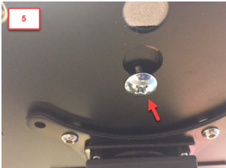
Tighten bottom screw into key-hole
