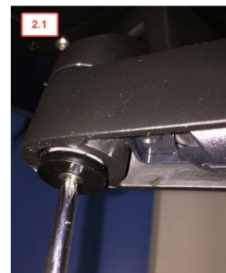
Attach tray to arm and attach washer under arm to tray
