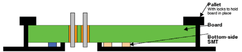
Figure 1. Selective solder pallet with a board.
