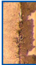
FIGURE 1: Failing open resistor area with visible crystalline growth.
