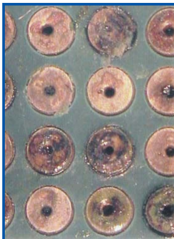
FIGURE 1: No-clean flux boards before rescue cleaning ...
