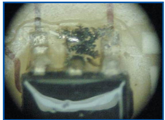
FIGURE 1: NTF returns are rising, the result of contamination stemming from board, component and assembly chemical processes.
