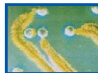
FIGURE 2: Copper sulfate corrosion.
