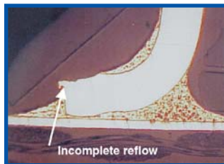
FIGURE 2: Cross-section of an SOIC termination.
