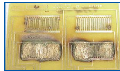
FIGURE 1: Thermally overstressed HASL boards processed with selective pallet soldering.
